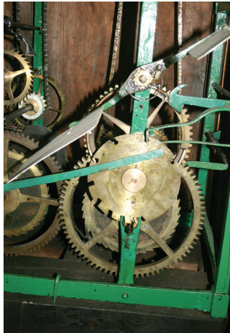
The clock's hourly stike control
