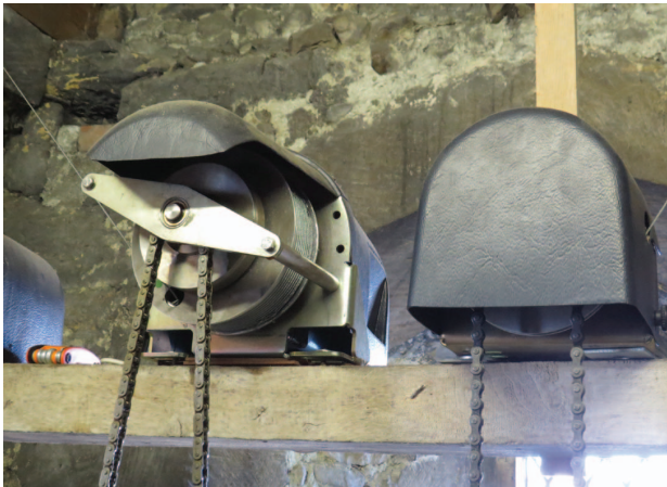
Electric winding mechanism for the clock
