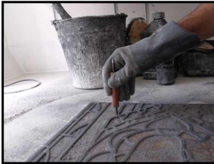
Waterproofing the glazing, application, drying, picking to remove the excess
